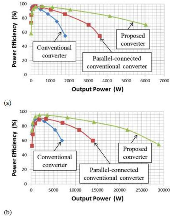
**Fig. 6:** Simulated power efficiency as a function of output power: (a) 1/2x step-down and (b) 2x step-up.
