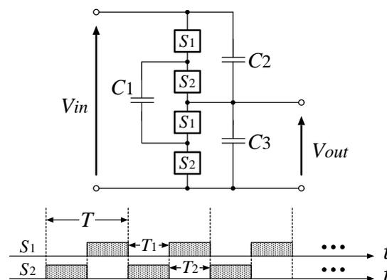
**Fig. 1:** Conventional SC AC-AC converter.
