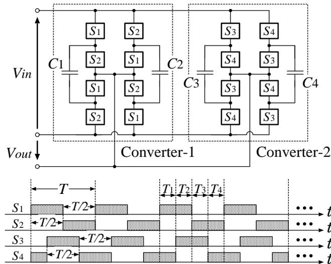
Fig. 2: Proposed SC AC-AC converter.
