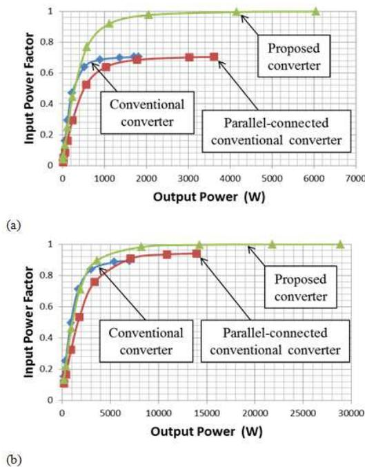
**Fig. 7:** Simulated input power factor as a function of output power: (a) 1/2x step-down and (b) 2x step-up.
