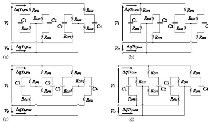
**Fig. 4:** Instantaneous equivalent circuits: (a) State- $T_1$ , (b) State- $T_2$ , (c) State- $T_3$  and (d) State- $T_4$ .
