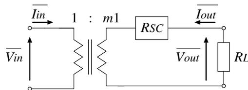
Fig. 3: Four-terminal equivalent model.
