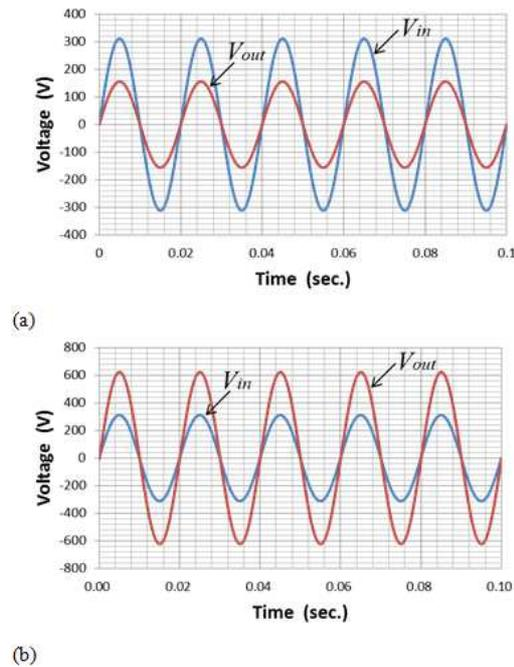
**Fig. 5:** Simulated output voltage: (a) 1/2x step-down and (b) 2x step-up.
